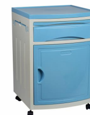
Model: YL-B1603 Bedside Cabinet Dimensions: 400 × 500 × 620mm 1. Cabinet Body: Made of electrolytic steel plate (thickness 1.0mm). 2. Main structure combines 2.0mm electrolytic steel plate and 2.0mm steel pipe. ; 3. Cabinet door and drawer feature hidden handles, formed by integrated bending. 4. Hinges:Hydraulic soft-closing mechanism. 5. Surface Treatment:Electrostatic epoxy resin powder coating.
