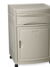
Model: YL-B1603 Bedside Cabinet Dimensions: 400 × 500 × 620mm 1. Cabinet Body: Made of electrolytic steel plate (thickness 1.0mm). 2. Main structure combines 2.0mm electrolytic steel plate and 2.0mm steel pipe. ; 3. Cabinet door and drawer feature hidden handles, formed by integrated bending. 4. Hinges:Hydraulic soft-closing mechanism. 5. Surface Treatment:Electrostatic epoxy resin powder coating.
